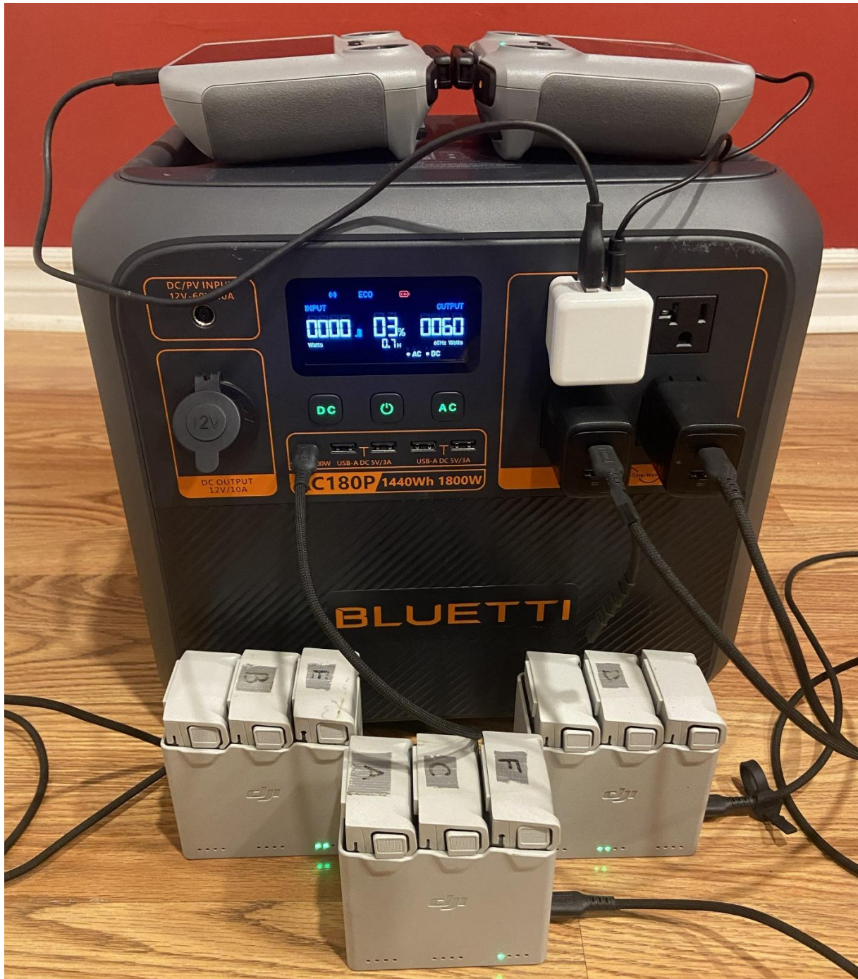
Figure 2-4. Charging station used in a study of painted turtle basking behaviour at Kenauk, Montebello, Québec, Canada, in 2025. The charging station consists of a Bluetti Portable Power Station powering three individual DJI Two-Way Charging Hubs with 30 W USB-C chargers, each charging three DJI Intelligent Flight Battery Plus units, for a total of nine batteries.
