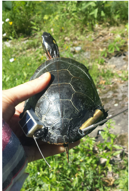
Figure 1. Accelerometer (left) and VHF transmitter (right) attached to the rear carapace margin of a Painted turtle. Photo by Anne-Christine Auge.
